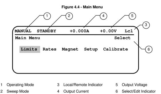
When in the menu system the top display line continues to update the status items shown. These items are described in Section 4.1. The Select/Edit (6) indicator appears on all the menu screens and indicates whether a field has been selected for edit. The arrow keys are used to highlight the desired option when Select is shown. Press the [Enter] key to select the item.
