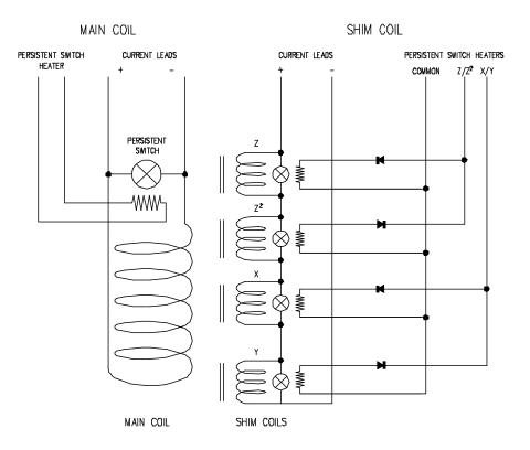
When the CS-4 Shim Supply Option is activated, the CS-4 uses its main current outputs to set the shim coil current. In shim mode the supply is software limited to a maximum current output. The current limit for each shim, the persistent switch heater current for each shim, and its overall status (enabled or disabled) is controlled through the menu system via the front panel keys.
