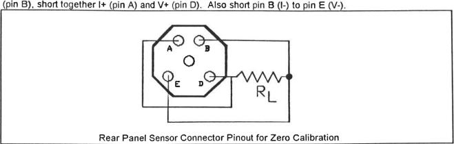
Reconnect the male sensor plug with the load resistor. Power ON. Adjust the ZERO potentiometer located on the rear panel until the digital display reads zero. If you have the TWO SENSOR Option follow the above procedure to adjust ZERO for the second sensor. Be sure to adjust the correct potentiometer that corresponds to the sensor selected on the front panel. The two sensors can be set independently of each other.
