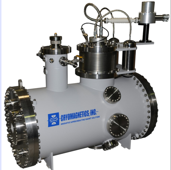
Recondensing Superconducting Magnet System
